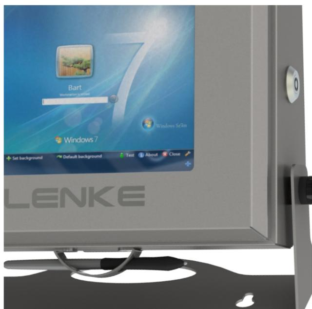
Lenke MI-3300 has Windows Operating System and works as a normal computer. It allows online access to production data, making constant monitoring and dynamic acting possible with the acquired information. As a standard computer, Lenke MI-3300 can have programs for production controlling and recording, as well as managing other industrial equipment.
